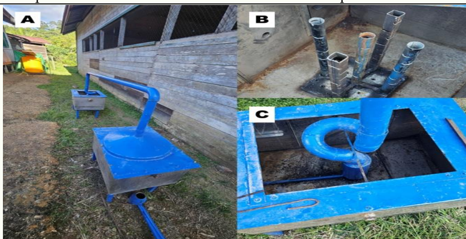
Figure 1. Portable pyrolysis unit donated to the Metut Village community for biomass conversion. (A) Fully assembled portable pyrolysis system showing the reactor and condensation unit used for the production of biochar and liquid smoke from woody biomass; (B) interior view of the pyrolysis reactor/combustion chamber where biomass feedstock is loaded and thermally decomposed under oxygen-limited conditions; and (C) dual-stage water-cooled spiral condenser used to condense volatile pyrolysis gases into liquid smoke.
